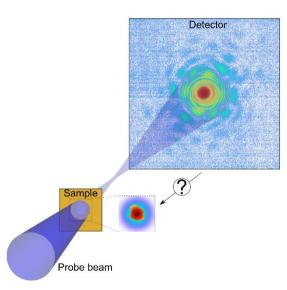
the sample, a precise 2D-reconstruction of the sample transmission is possible using an iterative algorithm. In my talk, I want to outline this exciting new technique that can in principle be used to image even very dynamical micro- and nanosamples.
